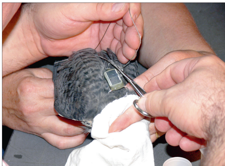
HOW IT'S DONE: A small wire harness is placed across the bird's chest. This holds the solar-powered 5g transmitter in place on the bird's back. An antenna runs along the bird's back. PICTURE: BIRDLIFE NORTHERN NATAL
