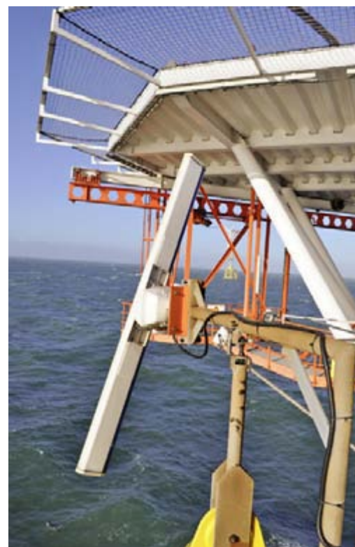
Vertical rotating marine radar device on FINO 1 for recording the intensity and height of migration.
